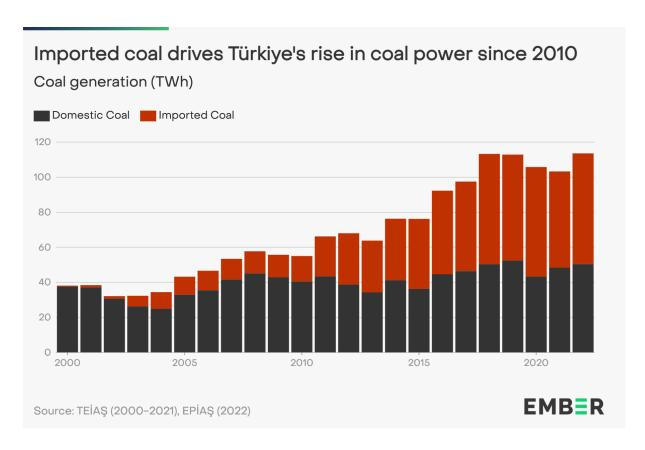
Imported coal has also pushed the upward trend in coal generation since 2010. In 2010, the share of imported coal generation was 7%, reaching 20% share in total power generation as of 2022. As of 2022, imported coal generation is over 4 times higher (63.2 TWh) than it was in 2010 (14.5 TWh).
